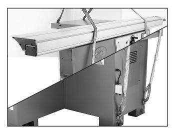
Figure 9. Lifting the saw base unit.
